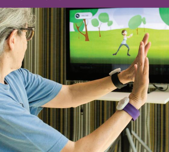
USER FRIENDLY BRACELET FEATURING AN ADVANCED INERTIAL MEASUREMENT UNIT AND BLUETOOTH SMART® CONNECTIVITY.
